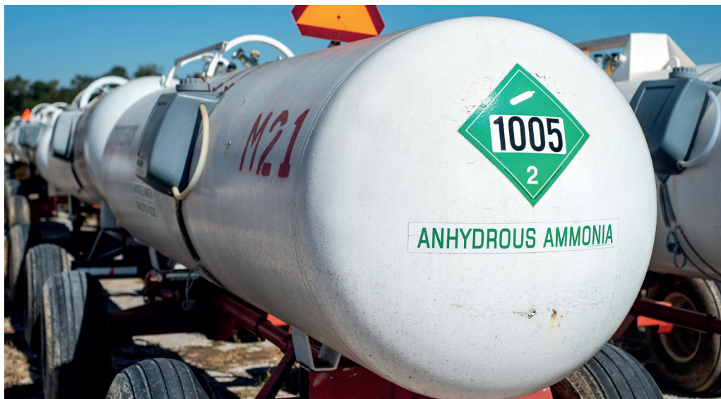
Anhydrous ammonia is transferred and stored as a liquefied, compressed gas.
