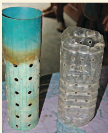
Perforated AWD-tube (left); locally adapted “pani pipe” (right).
